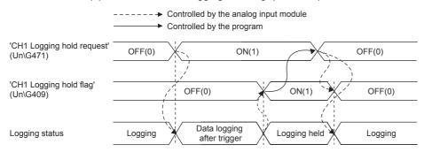
Logging does not stop when 'CH1 Logging hold request' (Un\G471) is changed on→off before ON (1) is stored in 'CH1 Logging hold flag' (Un\G409).
