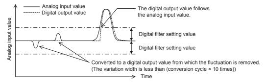
Digital filter requires the A/D conversion values for 23 times to remove the fluctuation which is smaller than the digital filter setting value. Therefore, when using the digital filter, the first digital output value is updated at the timing when the A/D conversion values for 23 times are completed.
