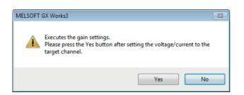
**8.** Input the Gain value voltage "5 V" to the terminal of the target channel (CH1) and click the [Yes] button.
