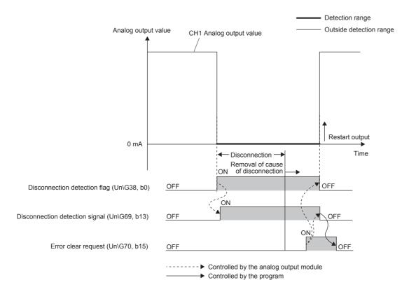
• Operation when 'Disconnection detection automatic clear enable/disable setting' (Un\G304) is Enable
