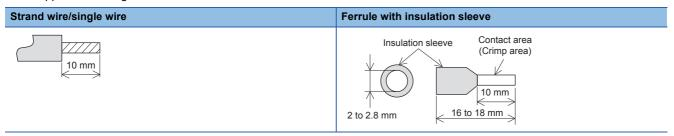
The following table shows wire ferrules and tools for wire ferrules compatible with the terminal block. Use of items other than these may result in not being able to remove the wire ferrule, so carefully check that the wire ferrule can be unplugged. <Reference product>
