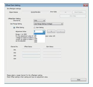
**4.** Specify the channel (CH1) and offset/gain setting used to perform the offset/gain setting.
