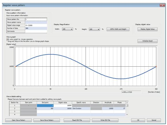
The created wave output data need to be written, as module extension parameters, to the CPU module or SD memory card.
