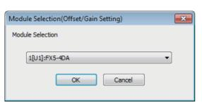
**2.** Select the target module for the offset/gain setting, and click the [OK] button.
