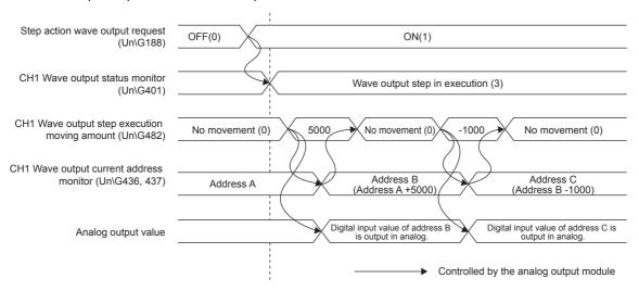
By turning 'Step action wave output request' (Un\G188) OFF (0)  $\rightarrow$  ON (1), change the status to Wave output step execution in progress. By setting the value in 'CH1 Wave output step action movement amount' (Un\G482) during wave output step execution, control moves to the address of the wave data to be subjected to the output test. For the value in 'CH1 Wave output step action movement amount' (Un\G482), set the amount by which to move it from the address of the current wave data.
