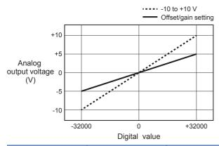
User rangeDigital valueResolutionRemarks-5 to +5 V-32000 to +32000321.5 μV(Gain value - Offset value) = 5 V<br/>As the result of (Gain value - offset value) is < 10 V, the maximum resolution is applied.</td>
