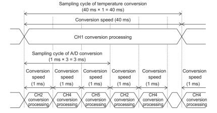
Conversion processing of A/D input range of module
