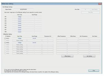
**4.** Mark the checkbox of the channel (CH1) where offset and gain values are to be set.
