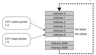
The head pointer does not change until CH1 Logging data (Un\G10000 to Un\G19999) becomes full after the logging start (fixed to 0).
