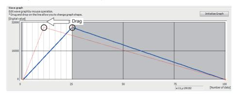
The end point position can be adjusted also by changing the "End point" and "Digital value" values in "Wave detail setting".
