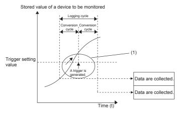
(1) The data at the timing when a trigger is generated is not stored in the buffer memory area.
