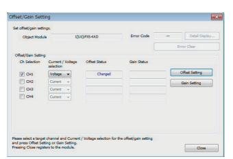
**6.** Input the offset value voltage "0 V" to the terminal of the target channel (CH1) and click the [Yes] button.
