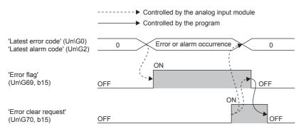
'Error flag' (Un\G69, b15), 'Latest error code' (Un\G0), and 'Latest alarm code' (Un\G2) are cleared at the timing when 'Error clear request' (Un\G70, b15) turns off→on.
