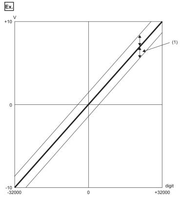
digit: Digital value V: Analog output value (V) (1): Fluctuation range
