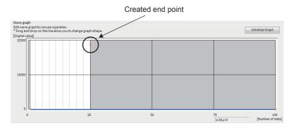
To delete it, move the mouse pointer to the terminal point and select "Delete End Point" from the right-click menu. Once the mouse pointer moves to the terminal point, its displayed shape changes to +.
