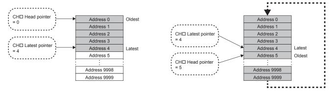
The head pointer does not change (fixed to 0) until CH1 Logging data (Un\G10000 to Un\G19999) becomes full after the logging start. (fixed to 0).
