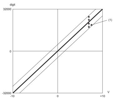
digit: Digital output value V: Analog input voltage (V) (1) Fluctuation range
