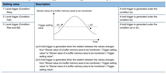
• Set a value where a hold trigger is generated to 'CH1 Trigger setting value' (Un\G542).
