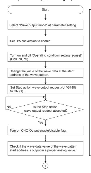
Example of executing a CH1 Analog output test
