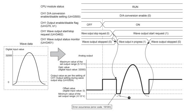
• If an attempt is made to output a value below the minimum value of the output range, the analog output value will be the minimum value of the output range.
