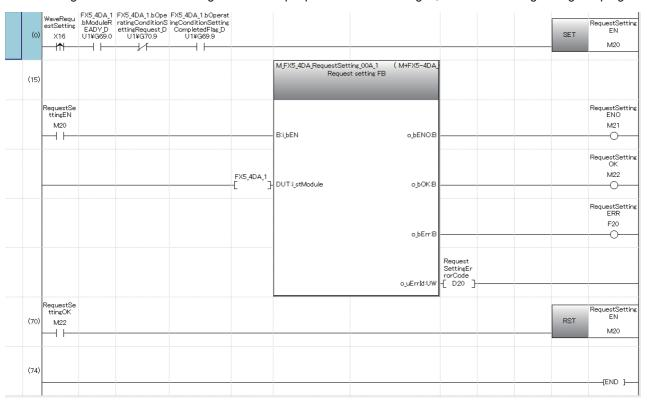
• Example of wave output star processing program This program example starts the CH1 wave output.
