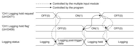
Logging does not stop when 'CH1 Logging hold request' (Un\G471) is changed from on  $\rightarrow$  off before ON (1) is stored in 'CH1 Logging hold flag' (Un\G409).
