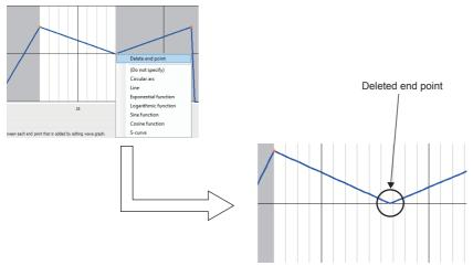
4. Set the wave between terminal points in the right-click menu or "Wave Specification" in "Wave Detail Setting".
